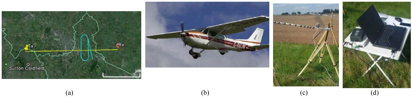
Figure 8 – Trials topology on Google Earth (a); Cessna 172 ultralight aircraft (b); receiver DVB-T and DAB antennas (c); USRP and the laptop (d).
