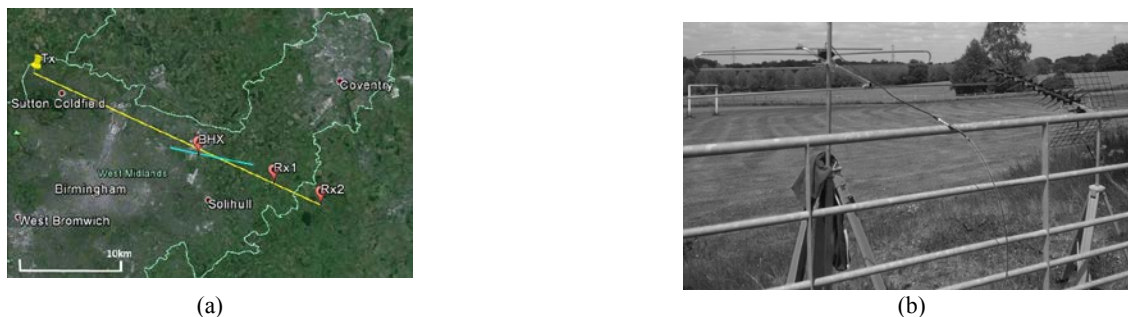
Figure 6 – Trials topology shown in Google Earth [25] (a), receiver Rx1 site at 6km (b) distance from crossing point, with FM and DVB-T antennas.
